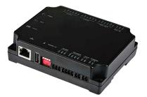
C2-260 is an IP-based two doors mini control panel. It supports TCP/IP communication through LAN or WAN network, and RS485 communication which allows extension to RS485 devices like DM10, AUX485, WR485. The series is a perfect match for the web-based software ZKBioAccess to provide RFID/Biometric Security solution. C2-260 can control two doors by default. It can extend to 8 DM10s at most that it can support up to 10 doors.
